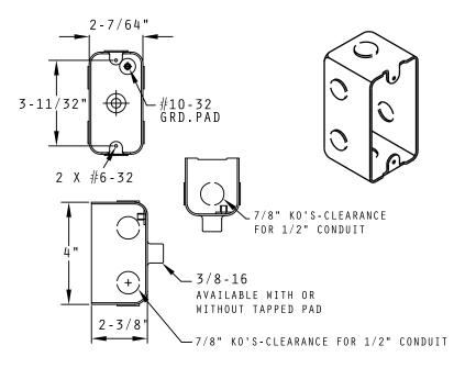
DRAWN 2X4 RECTANGULAR UTILITY BOXES ARE AVAILABLE WITH WELDED STUDS FOR EASY MOUNTING TO THE SHIP'S BULKHEAD. STEEL BOXES ARE ELECTROGALVANIZED.
